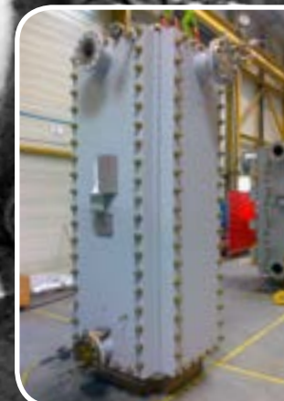
CLIENT/ USER: ENI SPA/ SANNAZZARO DE BURGONDI -ITALY Size / Weight/ Design Pressure: 750x750 N° 450 Plates H.3016/13900Kg/15 Bar.g. PLATE TYPE AND MATERIAL: WELDED PLATE/ASTM A240 TP 316L
