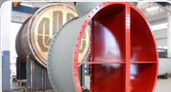
Client/User: Ge Oil & Gas / BRAHMAPUTRA CRACKER & POLYMER LTD Tema Type/Size/Weight/Design Pressure: CONDENSER / 2470/3055x5670 / 68000 Kg / 7,35 Bar.g Tube Type/Material: Bare tubes / ASTM B111 UNS C70600
