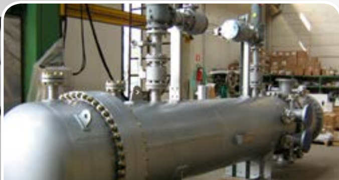
Client/User: K.O.C. – KUWAIT Tema Type/Size/Weight/Design Pressure: AFS / 940x4877 / 11500 Kg / 33,1 Bar.g Tube Type/Material: Bare Tubes / ASME SB163 UNS N08825
