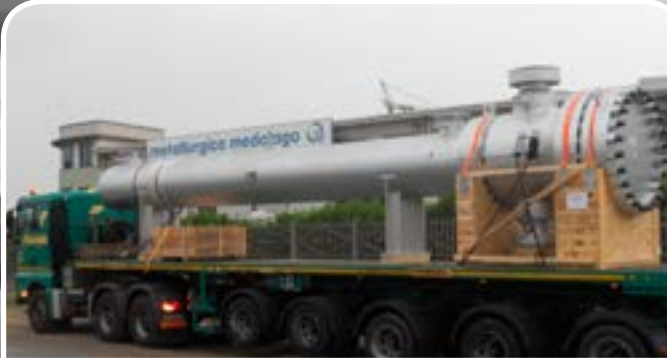
Client/User: Ge Oil & Gas / NUOVO PIGNONE Tema Type/Size/Weight/Design Pressure: DEU / 1000x9800 / 39000 Kg / 330 Bar.g Tube Type/Material: Bare "U" tubes / ASTM A213 TP.304L
