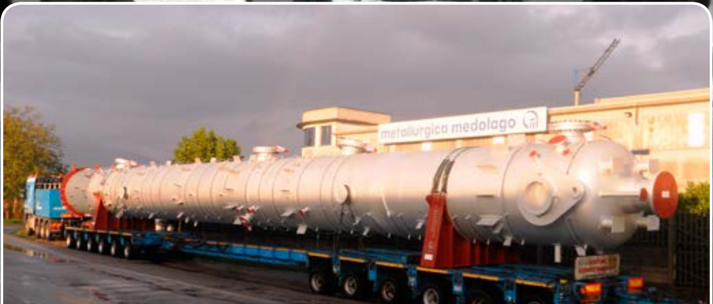
Client/User: P66 / HUMBER REFINERY - UK Size/Weight/Design Pressure: ID. 2210 x TL.@TL. 27356 / 62500 Kg / 3,4 Bar.g Material: ASTM A516 GR.60 + A240 TP.316L CLAD
