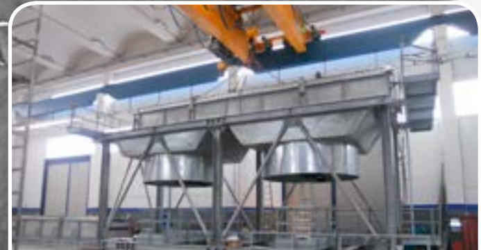
Client/User: HELLENIC PETROLEUM / ASPROPYRGOS - GREECE API661 Type/Plot Plan/Weight/Design Pressure: COVER / 4200x10970 / 37000 KG / 9 Bar.g Tube Type/Material: EMBEDDED Fin Tubes / ASTM A179
