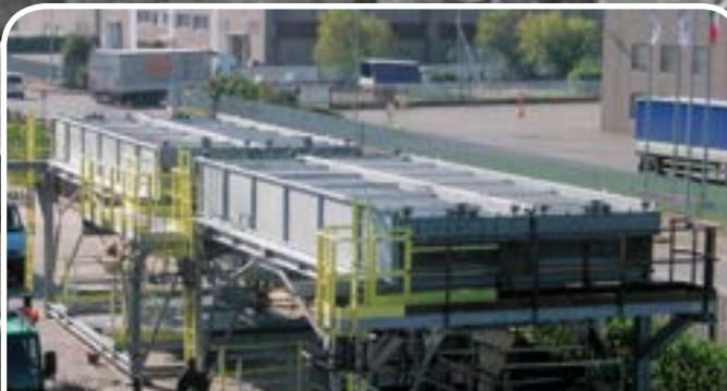
Client/User: RAFFINERIA ISAB IMPIANTI SUD PRIOLO - ITALY API661 Type/Plot Plan/Weight/Design Pressure: COVER / 4800x9144 / 26500 kg / 2 Bar.g Tube Type/Material: EMBEDDED Fin Tubes / ASTM A179
