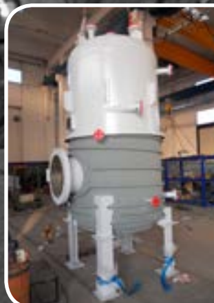
Client/User: ENI SPA / POLIMERI EUROPA RAVENNA PLANT – ITALY Size/Weight/Design Pressure: ID. 1400 x TL.@TL. 2200 / 2620 Kg / 17 Bar.g Material: ASTM A516 GR.60
