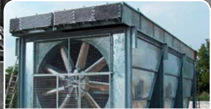
Client/User: AIRFINS LTD / DRESSER RAND – AHMEDABAD INDIA API661 Type/Plot Plan/Weight/Design Pressure: PLUG - Special Fans / 5400x13500x5500 / 30000Kg / 89,7 Bar.g Tube Type/Material: "KL" Fin Tubes / ASME SA214 Gr.M
