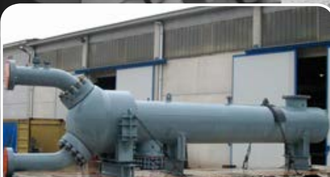
Client/User: GE Oil & Gas / Nuovo Pignone Tema Type/Size/Weight/Design Pressure: Special DEU / 1020x6100 / 30500 Kg / 620 Bar.g Tube Type/Material: Bare "U" tubes / ASTM A210 Gr.C
