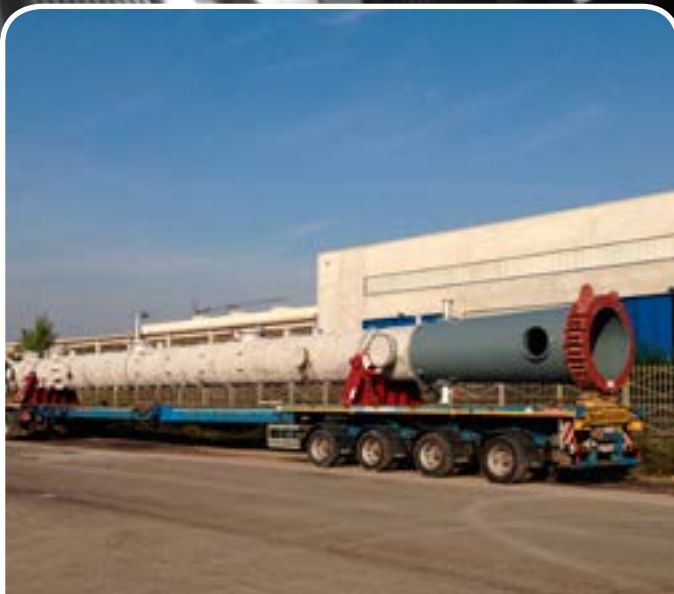
Client/User: P66 / HUMBER REFINERY - UK Size/Weight/Design Pressure: ID. 1296 x TL.@ TL. 23757 / 22700 Kg / 3,4 Bar.g Material: ASTM A 516 GR.60 / ASTM A516 GR.60 + A240 TP.316L CLAD
