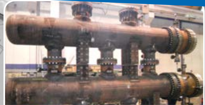
Client/User: PHILLIPS 66 / HUMBERSIDE – UK Tema Type/Size/Weight/Design Pressure: AXU / 762x4877 / 8413 Kg / 150 Bar.g Tube Type/Material: Bar "U" Tubes / ASTM A179
