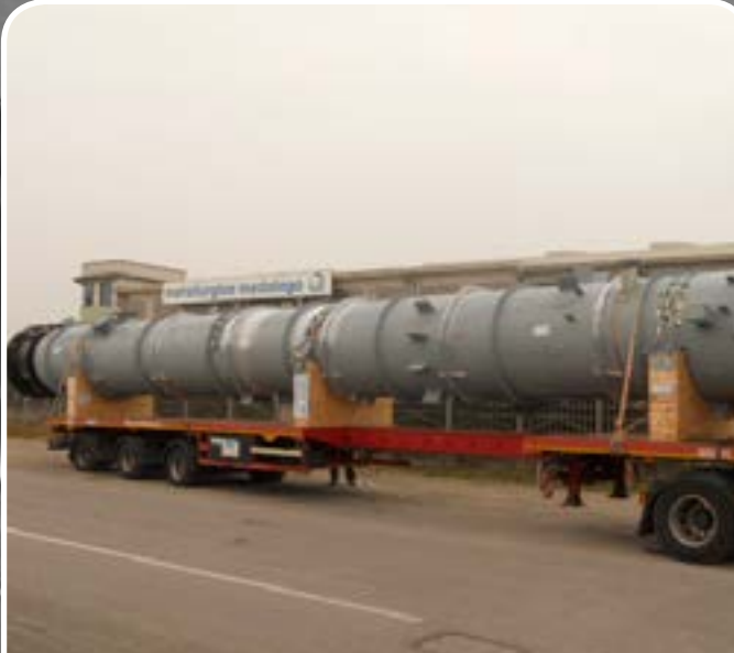
Client/User: ENI SPA / RAFFINERIA DI MILAZZO - ITALY Size/Weight/Design Pressure: ID. 1650 x TL. 8700 / 15000 Kg / 3,5 Bar.g Material: ASTM A516 GR.60 + A240 TP.316L
