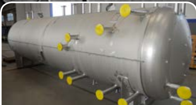
Client/User: SIRTEC NIGI / K.O.C KUWAIT Size/Weight/Design Pressure: ID. 1600 TL.@TL. 5800 / 5800 Kg / 10 Bar.g Material: ASME SA240 TP.316 L
