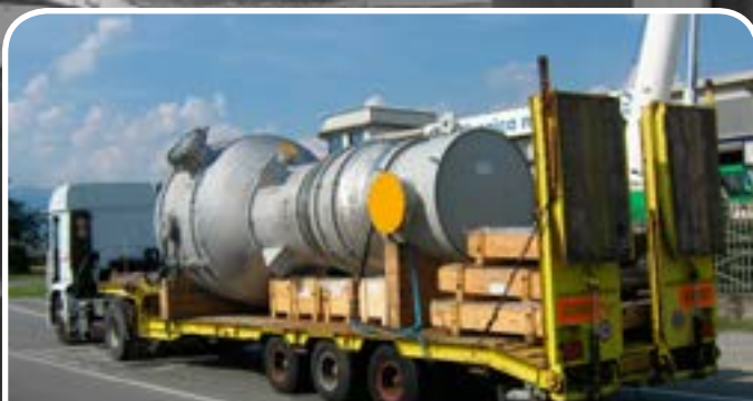
Client/User: AMMONIA CASALE / ZAKLADY AZOTOWE PULAWY " SPOLKA AKCYJNA - POLAND Tema Type/Size/Weight/Design Pressure: SPECIAL AEU / 1400/2500x3119 / 15500 Kg / 7 Bar.g Tube Type/Material: Bare "U" tubes / ASTM A213 TP.316L
