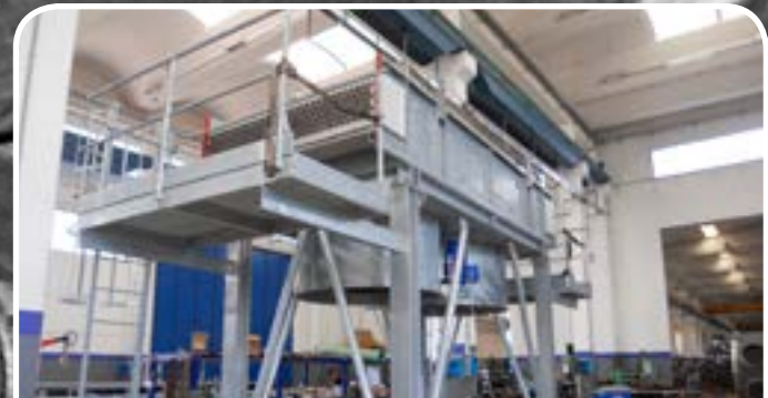
Client/User: GULF SPIC / KNPC MINA AL-AHMADI REFINERY – KUWAIT API661 Type/Plot Plan/Weight/Design Pressure: PLUG / 2500x4300 / 11500 Kg / 10 Bar.g Tube Type/Material: EMBEDDED Fin Tubes / ASME SA179
