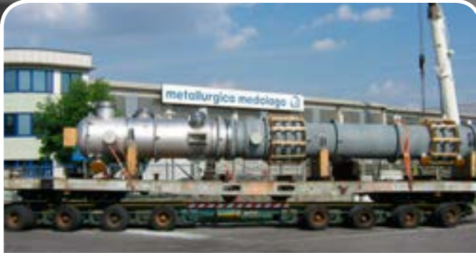
Client/User: AMMONIA CASALE / ZAKLADY AZOTOWE PULAWY " SPOLKA AKCYJNA - POLAND Tema Type/Size/Weight/Design Pressure: SPECIAL BEM / 1100x8093 / 30700 Kg / 34 Bar.g Tube Type/Material: Bare tubes / ASTM A213 TP.316L
