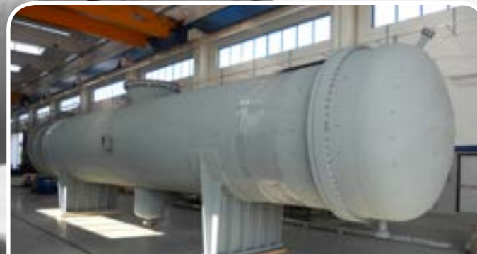
Client/User: KÖRTING AG / ZAO " ANTIPINSKY REFINERY " - RUSSIAN FEDERATION Tema Type/Size/Weight/Design Pressure: AXS / 1900x10500 / 65000 Kg / 10 Bar.g Tube Type/Material: Bare Tubes / ASTM A312 TP.316L
