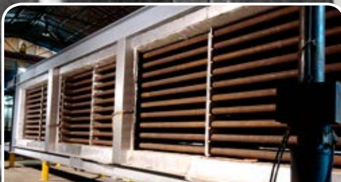
Client/User: IPSL LTD METHANOL HOLDING / POINT LISAS - TRINIDAD Size/Weight/Design Pressure: 3140x19710x4850 / 90000 Kg / 32,5 Bar.g Tube Tp/Mat.: Bar Tubes/ASTM A335 P11 - WELD. Fin Tubes/ASTM A335 P11 @ ASTM A 240-410
