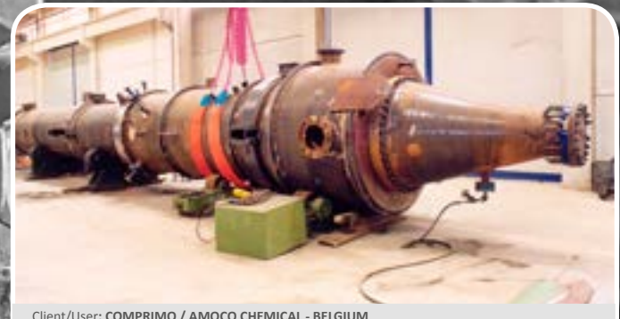
Client/User: COMPRIMO / AMOCO CHEMICAL - BELGIUM Tema Type/Size/Weight/Des. Pres.: SPCL FX TUBESHEET / 1550/1900x5500 / 25300 Kg / 20,7 Barg Tema Type/Size/Weight/Des. Pres.: SPCL FX TUBESHEET / 1280x7000 / 26000 Kg / 20,7 Barg Tube Type/Material: Bare Tubes WITH GRID BUFFLES TYPE / ASTM A179 Tube Type/Material: LOW FIN Tubes / ASTM A179
