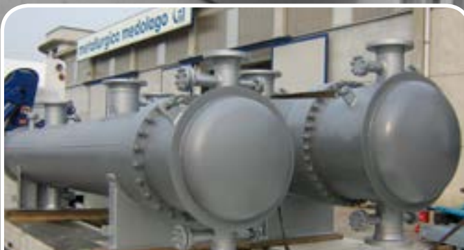
Client/User: PHILLIPS 66 / WHITEGATE REFINERY – IRELAND Tema Type/Size/Weight/Design Pressure: BHU / 896x6580 / 7800 Kg / 25,5 Bar.g Tube Type/Material: Bar "U" Tubes / ASTM A179
