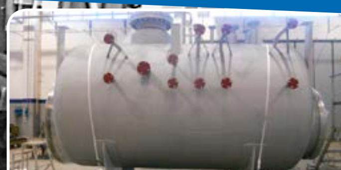
Client/User: P66 / HUMBER REFINERY – UK Type/Size/Weight/Design Pressure: WHB / 4256x2450 / 27700 Kg / 30,34 Bar.g Tube Type/Material: Bar Tubes / ASTM A192
