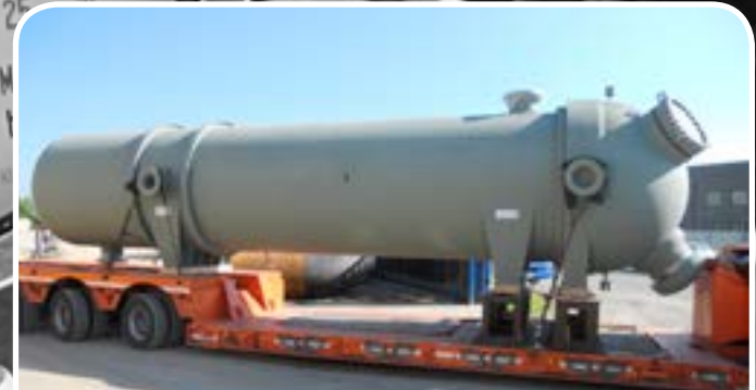
Client/User: METHANOL HOLDING TRINIDAD LTD / POINT LISAS - TRINIDAD Tema Type/Size/Weight/Design Pressure: DEU / 1850x7200 / 42200 Kg / 88,25 Bar.g Tube Type/Material: Bare "U" Tubes / ASTM A213 TP.304
