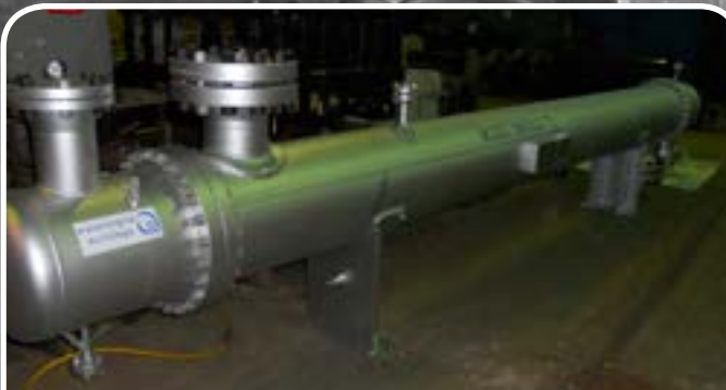
Client/User: QAFCO / MESAIEED Tema Type/Size/Weight/Design Pressure: BEM / 16 "x4877 / 1900 Kg / 52 Bar.g Tube Type/Material: Bar Tubes / ASME SB668 UNS N08028 (SANICRO 28)
