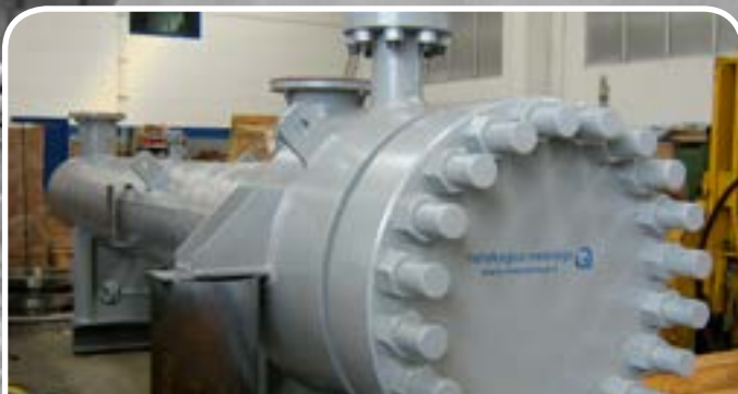
Client/User: Ge Oil & Gas / BOREALIS STENUNGSUND PLANT - SWEDEN Tema Type/Size/Weight/Design Pressure: DEU / 660x5300 / 12800 Kg / 334 Bar.g Tube Type/Material: Bare "U" Tubes / ASTM A210 Gr.A1
