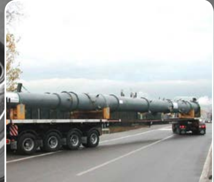
Client/User: KNPC / SHUAIBA REFINERY - KUWAIT Size/Weight/Design Pressure: ID. 1072/781 x TL.@TL. 28194 / 18400 kg / 9,65 Bar.g Material: ASME SA516 Gr.70 + SA240 TP.304L CLAD / ASME SA516 GR.70 + HASTELLOY C22 CLAD
