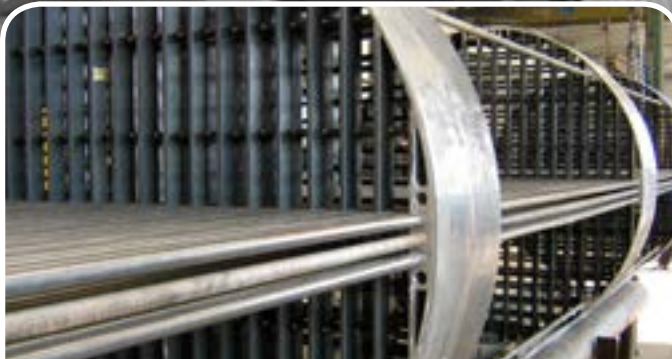
Client/User: DUPONT INTERNATIONAL SA/ RAFFINERIA DI MILAZZO - ITALY Tema Type/Size/Weight/Design Pressure: Spare Bundle / 1610x8528 / 23500 kg / 6,9 Bar.g Tube Type/Material: SPECIAL Bare " U" BUNDLE WITH GRID BUFFLE TYPE / ASTM A179
