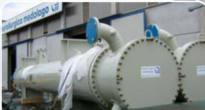
Client/User: Ge Oil & Gas /KNPC – KUWAIT Tema Type/Size/Weight/Design Pressure: AES / 711x6706 / 6550 Kg / 12 Bar.g Tube Type/Material: Bare Tubes / ASME SA179
