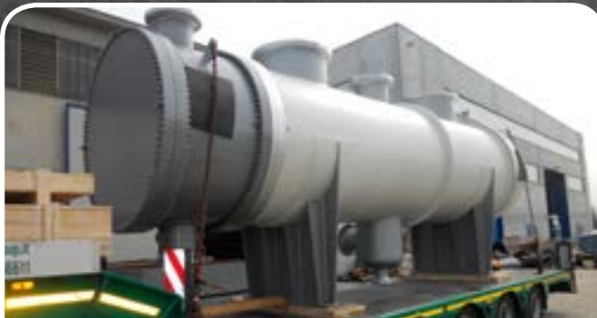
Client/User: KÖRTING AG / OMV PETROM S.A. PETROBRAZI REFINERY – ROMANIA Tema Type/Size/Weight/Design Pressure: AES / 1810x6000 / 35000 kg / 7 Bar.g Tube Type/Material: Bare Tubes / ASTM B111 UNS C71500
