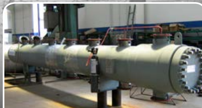
Client/User: METHANOL HOLDING TRINIDAD LTD / POINT LISAS - TRINIDAD Tema Type/Size/Weight/Design Pressure : DXU / 750x6500 / 11000 Kg / 126 Bar.g Tube Type/Material: Bare "U" tubes / ASTM B163 UNS N04400
