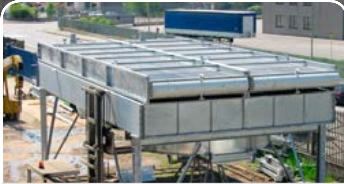
Client/User: AIRFINS LTD / GNPOC – SUDAN API661 Type/Plot Plan/Weight/Design Pressure: BONNET / 24000x12144 / 88000 Kg / 12 Bar.g Tube Type/Material: "KL" Fin Tubes / ASME SA179
