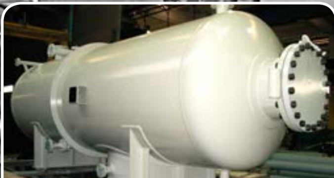
Client/User: AGIP PETROLI / PRIOLO PLANT – ITALY Size/Weight/Design Pressure: ID. 1400 x TL. 4000 / 3900 Kg / 10 Bar.g Material: ASTM A516 GR.65
